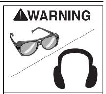
Operating this stapler can propel objects into the air, causing immediate eye damage. To protect yourself, always wear American National Standards Institute (ANSI) approved safety glasses or goggles when operating this equipment. In addition, this stapler discharges at 85-90 decibels. To protect your hearing, always wear ANSI approved ear protection when operating this stapler.
